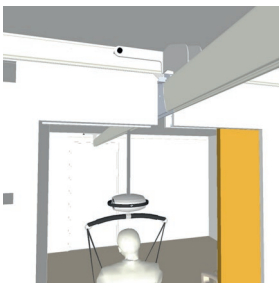
Room to room with 5.4 inch track and door connectors.
