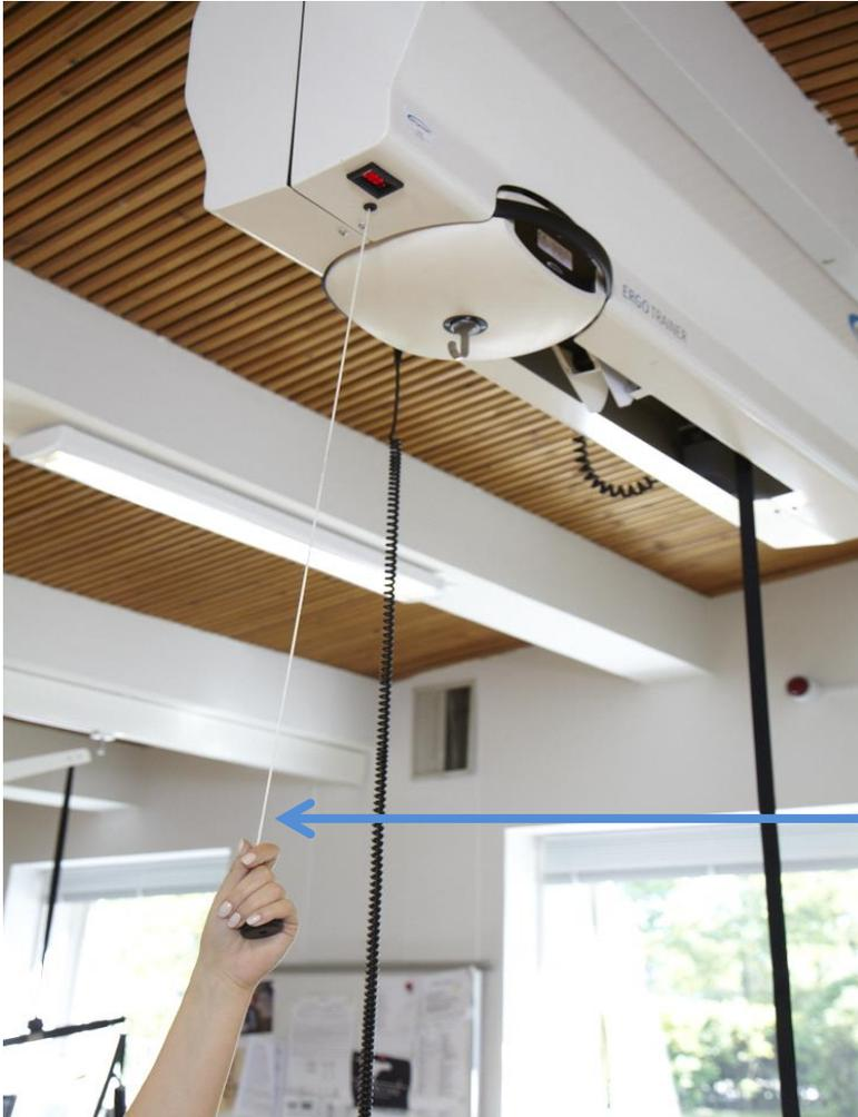
Pull cord to lock or to release the Ergo Trainer into desired position on the track.
