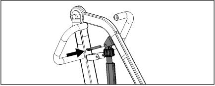
**Step 10**: Insert the spreader bar into the tube on the boom as follows. Align the holes and secure the spreader bar using a pin and retainer ring.
