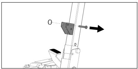
**Step 8**: Move the boom out of the way, and install the lower end of the actuator to the mast using a pin and retaining ring as follows.
