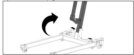
Step 5: Insert the pin to secure the mast.
