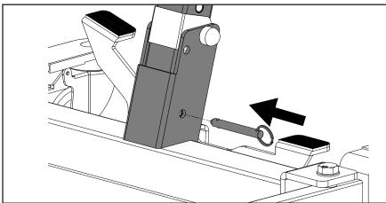
**Step 6**: Remove the pin that is securing the boom.
