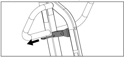
Step 7: Remove lower actuator pin on the mast.
