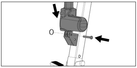
**Step 9**: Install the upper end of actuator to the boom by reinsert the quick release pin to secure it.
