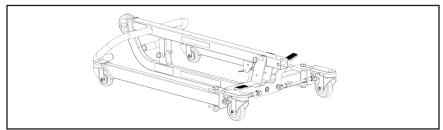
**Step 2**: Secure the stand to the mast. Hold the nut on its side with two fingers. Align the nut and the hole on the stand bracket with the lower hole on the mast. Make sure the tab on the stand bracket sit in the top hole on the mast, and insert the screw to the nut as follows. Use the EZ-Tools to tighten the screws.
