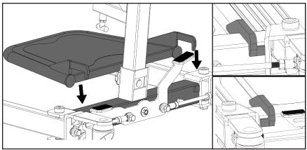
**Step 7**: Install the kneepad frame with the plastic U washer to the kneepad. Choose one of the three holes on the tube depending on the desired kneepad height. Then secure it using bolt, nut and washers as follows.
