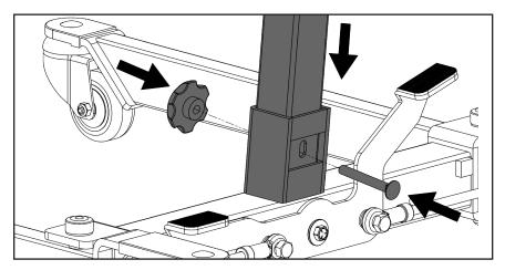
**Step 3**: Insert the boom to the mast and secure it using the bolt and threaded knob as follows.
