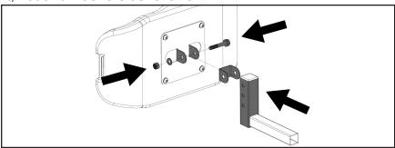
**Step 8**: Pull the depth adjustment handle down and insert the kneepad frame into the receiving tube located on the mast. Release the handle and continue sliding the kneepad frame until the handle clicks to ensure kneepad frame is locked in place.
