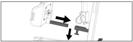
**Step 9**: For SA400HE model, refer to "Quick Setup Guide to TiMotion Electronics" to install the controller.
