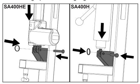
**Step 5**: Insert the upper end of the actuator (SA400HE) or the hydraulic pump (SA400H) to the bracket on the boom and secure it using a pin and retaining ring as follows.
