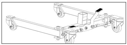
**Step 2**: Insert the mast and secure it using the bolt and threaded knob as follows.
