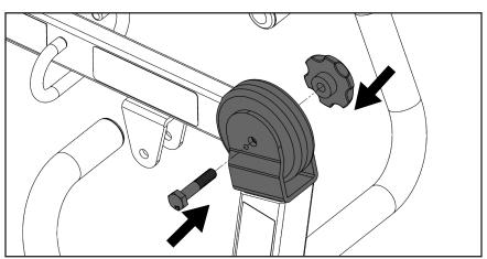
**Step 4**: Insert the lower end of the actuator (SA400HE) or the hydraulic pump (SA400H) to the bracket on the mast and secure it using a pin and retaining ring as follows.
