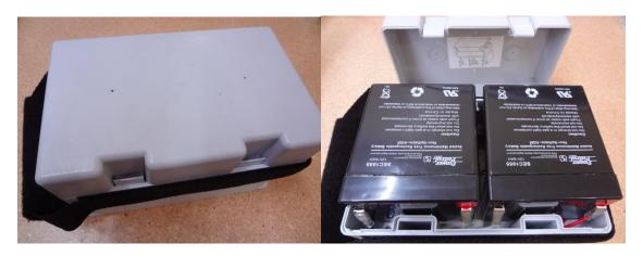
Place the control box on a flat surface with the recess latches facing up. Press both latches and pull up the cover.
