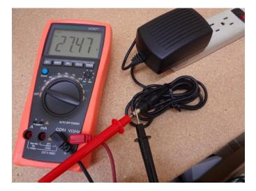
The output of the charger can be checked using a volt meter. If the output of the charger is below 26.5VDC, the charger is defective and needs to be replaced.
