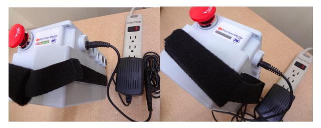
Plug the external charger to a power source at one end and the other end to the control box. Turn the red reset switch clockwise and let it pops up and the Indication lights will be on. If the lights are not on when the reset switch is in the UP position, the charger is defective.
