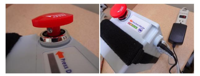
Make sure the reset switch is in UP position. The lift won't work if the switch is in DOWN position.
