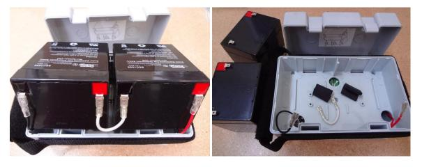
Pull out the batteries carefully and disconnect the connectors at the battery terminals.
