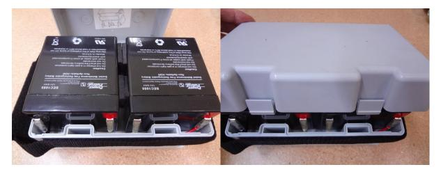
Put the new batteries and foams in place and re-connect the battery connectors at the terminals. Then put the cover in a slight angle and snap the latches in.
