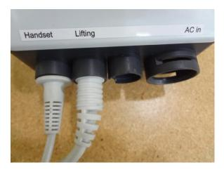
Make sure the two connectors are fully inserted to the control box as shown.
