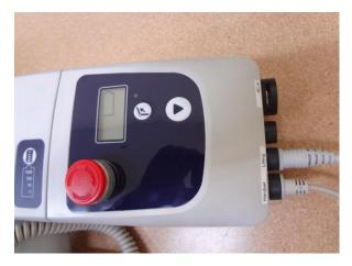
Make sure the red button is in UP position. The lift won't work with the button in DOWN position.
