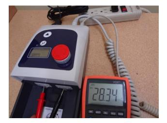
Charging output can be measured at the two battery contact points with the power cord plug-in. Voltage should be above 26.5VDC.
