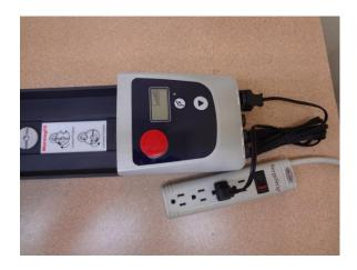
With the power cord plug-in without the battery pack, the green indicating light will be on and the LCD display will show 4 bars. If not, the cord is defective.
