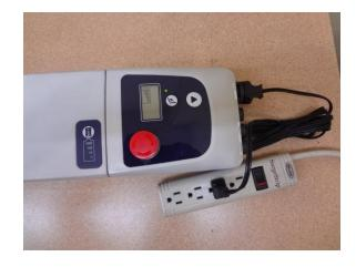
With the power cord plug-in with the battery pack, the green indicating light will be on and LCD display will show 4 flashing bar. If not, the charging system is defective or the battery pack doesn't make good contact with the control box.
