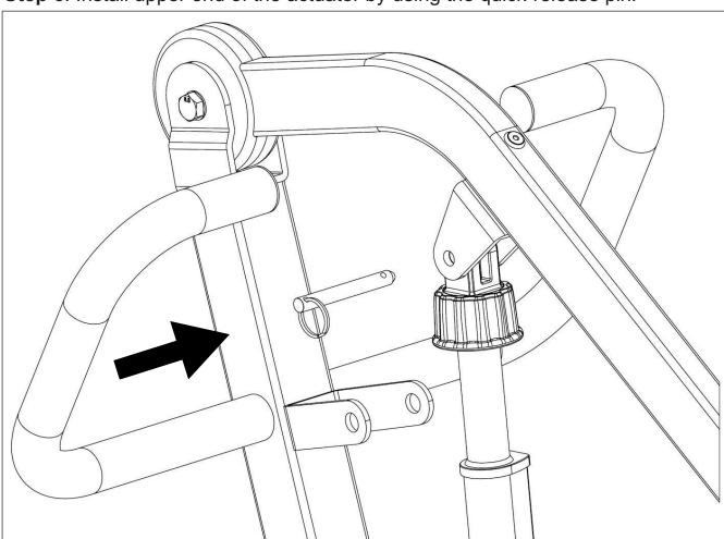
**Step 6**: Install upper end of the actuator by using the quick-release pin.
