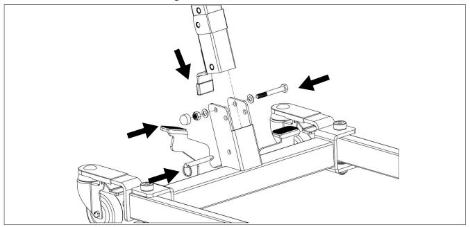
**Step 4**: Attach the joint cover to the boom as shown. Insert the boom to the mast and secure it using the hardware. Use wrenches to tighten the hardware.
