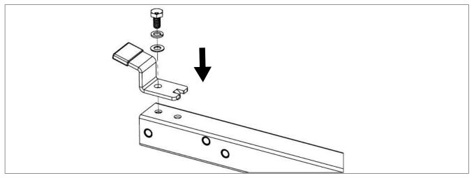
**Step 3**: Lock the rear casters on the base and insert the mast into the base bracket by aligning the holes. Secure the mast to the base using the hardware as shown. Use wrenches to tighten the hardware.
